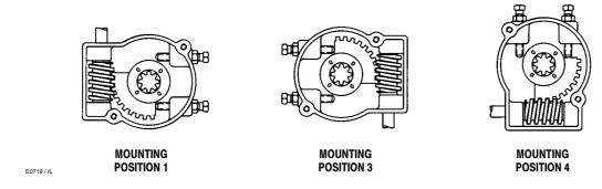
Figure 5. Reverse Acting Mounting Positions (shown in the closed position)
